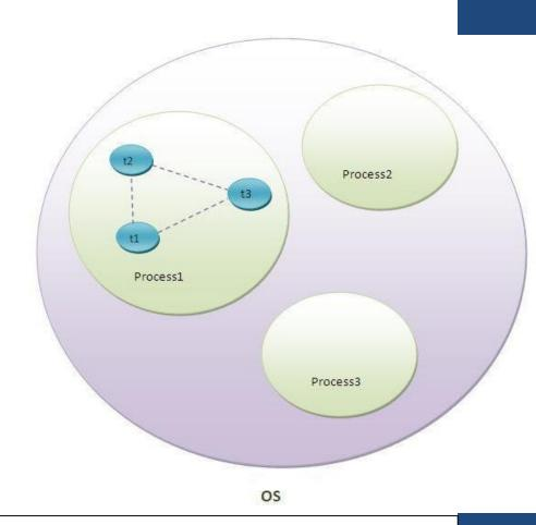
In this figure, thread is executed inside the process. There can be multiple processes inside the OS and one process can have multiple threads.
