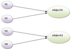
In case of synchronized method and synchronized block there cannot be interference between t1 and t2 or t3 and t4 because t1 and t2 both refers to a common object that have a single lock.
