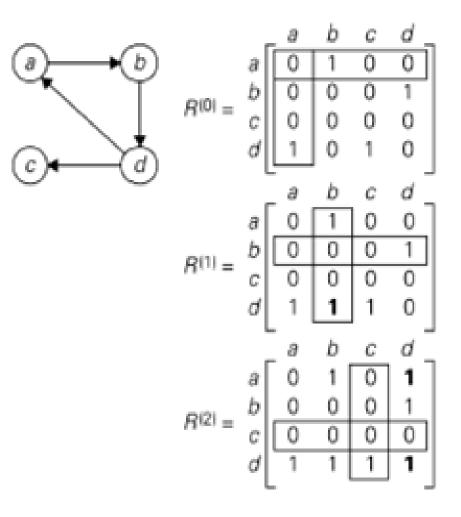
Ones reflect the existence of paths with no intermediate vertices (R<sup>(0)</sup> is just the adjacency matrix); boxed row and column are used for getting R<sup>(1)</sup>.
