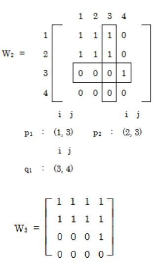
Finally,  $W_3$  has 1's in locations 1, 2, 3 of column 4 and no 1's in row 4, so no new 1's are added and  $MR_{\infty} = W_4$ =  $W_3$ .
