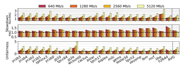
The figure above shows the slowdown experienced, as well as unfairness index, of RNG vs non-RNG applications over a wide variety of benchmarking formats, as well as a range of different throughput speeds.
