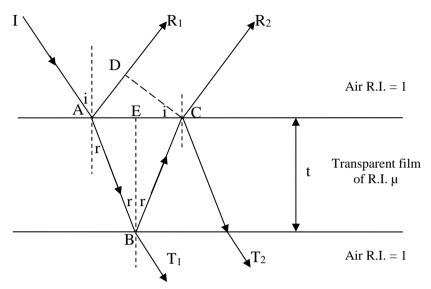
The optical path difference between the interfering rays  $R_1$  and  $R_2$  is given by
