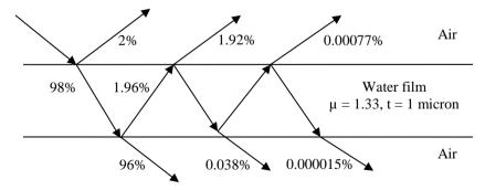
We consider a parallel beam of light incident on a thin transparent film of uniform thickness "t" and refractive index " $\mu$ ". As shown in the figure, multiple reflections would take place. However, much of the incident light will get transmitted through the film. If we have a soap bubble for example, by taking the R.I. to be 1.33, the amount of light reflected is nearly 2%. A part of light passing through the water film gets reflected from the second boundary.
