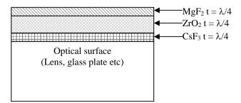
A single layer antireflection film is effective only at a certain wavelength and cannot totally reduce the reflection. Therefore, in practice, often multilayer films coatings are used. A three later coating system is widely used and effective over most of the visible spectrum coming from sunlight or lamps.
