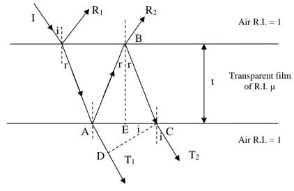
So, in this case, the optical path difference is given by
