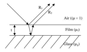
(a) Condition on refractive index: This condition says that the amplitudes of two rays  $R_1$  and  $R_2$  must be equal to obtain effective interference.
