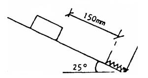
21. 20 N block slides with initial velocity 2 mls down an inclined plane on to a spring of modulus 1000 N/m for a distance of 1m. Find maximum compression of the spring neglecting and considering friction.
