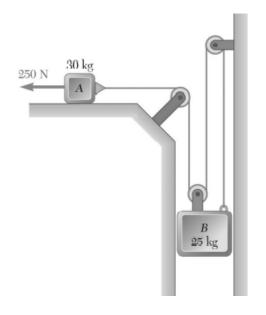
6. The system shown is at rest when a constant 250-N force is applied to block A. Neglecting the masses of the pulleys and the effect of friction in the pulleys and assuming that the coefficients of friction between block A and the horizontal surface are 0.25  $\mu$  s = and 0.20,  $\mu$ k = determine (a) the velocity of block B after block A has moved 2 m, (b) the tension in the cable.
