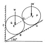
13. Two spheres, each of weight 1000 N and of radius 25 cm rest in a horizontal channel of width 90cm as shown in Fig. Find the reactions on the points of contact A, B and C. (Ans :  $R_A = R_C = 1333.33$ ,  $R_B = 2000$ ,  $R_D = 1666.67$ )
