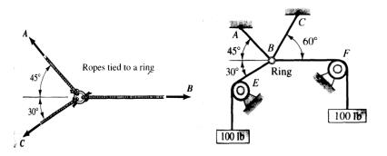
50. Find the tensile force in cables AB and CB. The remaining cable ride over frictionless pulleys E and F.
