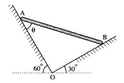
31. If the end B of the ladder of the rest against a wall find the reactions-at A and B
