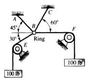
9. Find the force transmitted by wire BC. The pulley E can be assumed to be frictionless in this problem. (Ans : BC = 113.14, AB = 180, BD = 128.13)
