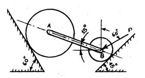
30. nA uniform bar AB of length L and weight W lies in a vertical plane with its ends resting on two smooth surfaces on OA and OB. Find angle  $\theta$  for equilibrium of bar.( Ans :  $\theta$ = 30°)
