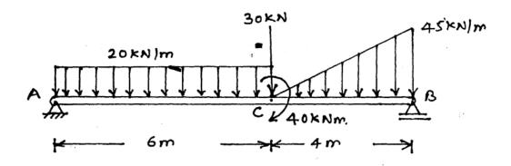
26. Calculate support reactions for the following beam.
