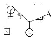
8. Find the tensile force in cables AB and CB. The remaining cable ride over frictionless pulleys E and F.( Ans : BC = 26.79, AB = 37.9)
