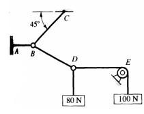
52. Find the tensions in the three cables connected to B. The entire system of cables is coplanar. The roller at F is free to turn without resistance.
