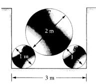
23. The roller shown in fig is of weight 1500N. What force T is necessary to start the roller over the block A?
