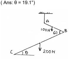
37. Determine the angle  $\theta$  & tensions in the cables AB & CD. (AB is horizontal) Wt of BC is w N.
