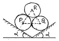
22. Cylinders A and B weigh 500 N each and cylinder C weighs 1000 N. Compute all contact forces.( Ans : 671, 447, 1000 )
