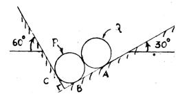
18. The roller shown in fig is of weight 1500 N . What force T is necessary to start the roller over the block A?( Ans : 1759.34 )
