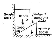
7. A block of mass 150 kg is raised by a 10° wedge weighing 50 kg under it and by applying a horizontal force at it as shown in figure. Taking coefficient of friction surfaces of contact as 0.3, find what minimum force should he applied to raise the block.
