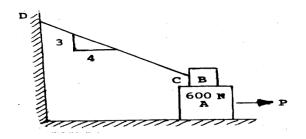
5. Find the value of load W so that the blocks A & B are just on the point of sliding.  $\mu$  between ground & block = 0.2.
