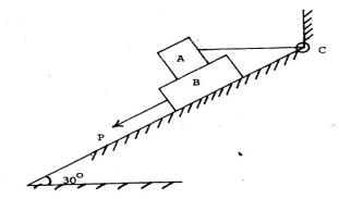
16. What should be the value of ' $\theta$ ' so that the motion of block 'A' impends down the plane? The coefficient of friction ' $\mu$ ' for all the surfaces is 1/3. Mass of A = 40 Kg & Mass of B = 13.5 Kg.
