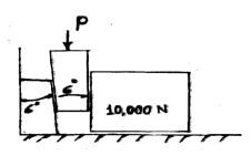
10. To raise a heavy stone block weighing 2000 N, the arrangement shown is used. What horizontal force P will be necessary to apply to the wedge in order to raise the block if the  $\mu$  for all continuous surfaces is  $\mu$  = 0.25? Neglect the weight of the wedge. (Ans: 1870)
