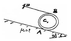
18. Determine the minimum weight W to prevent downward motion of the 1000 N body. Take  $\mu$ = 0.2 between the rope and the fixed drum and  $\mu$  = 0.3 for other surfaces of contact.(Ans :
