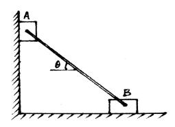
7. An non-homogeneous ladder as shown in the figure rests against a smooth wall at A and a rough horizontal floor at B. The mass of the ladder is 30 kg and is concentrated at 2 m from the bottom. The coefficient of static friction between the ladder and the floor is 0.35. Will the ladder stand in 60° position as shown ?
