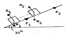
14. Find the tensions in the chords of the inclined plane system shown in figure.
