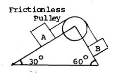
9. Find the value of  $\theta$  if the blocks A and B shown in fig. have impending motion. Given Block A = 20kg, Block B = 20kg &  $\mu$  = 0.25. (Ans:  $\theta$  = 28.08°)
