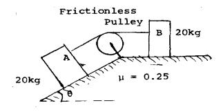
10. Determine the force P to cause motion to impend if the coefficient of friction for both blocks and the plane shown in fig. is 0.25. The force P and the ropes are parallel to the plane. The pulley is frictionless.
