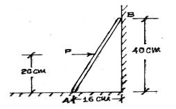
5. A weightless ladder of length in is resting against a smooth vertical wall and rough horizontal ground as shown in the figure .The coefficient of friction between ground and ladder is 0.25. A man of weight 500 N wants to climb up the ladder. Find how much distance along the ladder the man can climb without slip. A second person weighing 800 N wants to climb up the same ladder. Would he climb less than the earlier person? Find his distance covered. (Ans : 3.464 )
