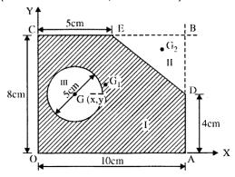
24. Determine the centroid for the shaded area as shown in figure. (Ans: X = 2.64, Y = 0.01)
