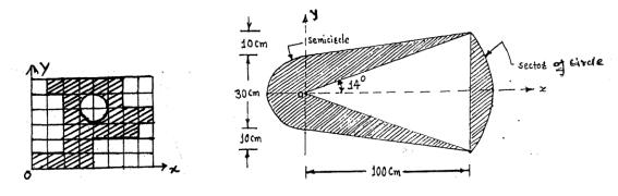
4. Calculate, numerically, the co-ordinates x and of the centroid C of the shaded area shown in figure. Each of the grid measures 10 mm x 10 mm.
