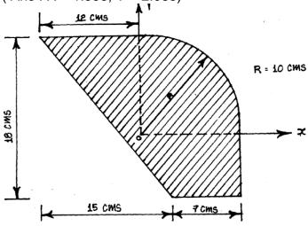
11. Determine the co-ordinate of centroid of the shaded portion shown in figure.
