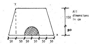
10. Determine the position of the centroid of the plane shaded area shown in figure.
