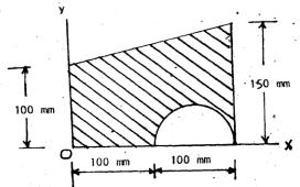
9. Locate the centroid fo the cross section shown in Fig. (Ans: Y = 99.48)
