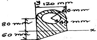
6. Determine the distance 'h'or which the centroid of the shaded area is as high above line AA as possible. Show that if the distance y of C.G. is maximum, 'y = h Shown in Figure. ( Ans: h = 612.57)
