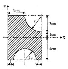
25. Determine the centroid for the shaded area as shown in figure. ( Ans : X = 4.823, Y = 8.16 )
