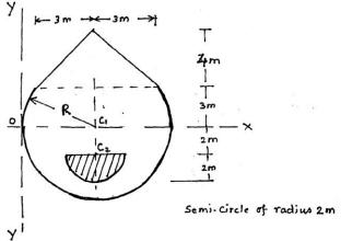
3. Calculate numerically centroid of the shaded area shown in Fig. ( Ans : X = 29.64 )
