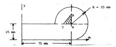
22. Determine depth of web of Tee-section, such that centroid of section coincides with AB axis. (Ans: h = 55.91)
