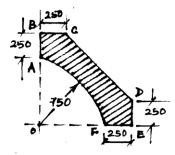
16. Determine the C.G of the following plane area shown in fig. (Ans: X = 54.86, Y = 18.46)
