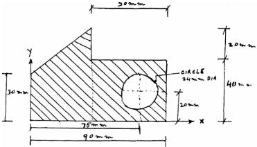
2. Find coordinates of centre of gravity for the following lamina. Please note that the shaded area is the opening in the lamina. (Ans: X = 4.243, Y = 0.7044)
