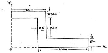
31. Find the centroid of the shaded area as shown in Fig. (  $\mbox{Ans}: X =$  - 19.33, Y = 93.02, )
