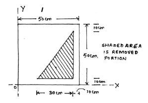
30. Find the centroid of the shaded area as shown in Fig  $\,$  (Ans : X = 13.55, Y = 10.4,)
