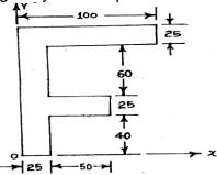
14. Locate the centroid of the shaded area in figure with respect to the co-ordinate axes as shown. (Ans: X = Y = 0.07446 a)
