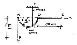
2. The figure below shows is formed of a thin homogeneous wire. Find the length '1' of portion CE of the wire for which the centre of gravity of the figure is located at C.
