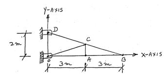
13. Find the length L of a portion of bent up wire shown in figure. The C.G. of a whole figure is at point 0.
