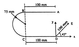
9. A uniform wire is bent into a shape shown in figure. Calculate the position of the C.G. (Ans : X = 10.29 , Y = 5.1 )
