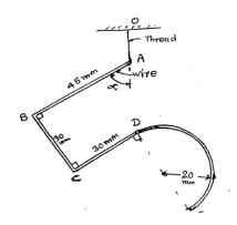
8. A uniform wire is bent into a shape shown in figure. Calculate the position of the C.G. (Ans: X = 77.065, Y = 67.6)
