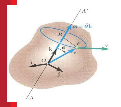
• Motion of a rigid body rotating around a fixed axis is often specified by the type of angular acceleration.
