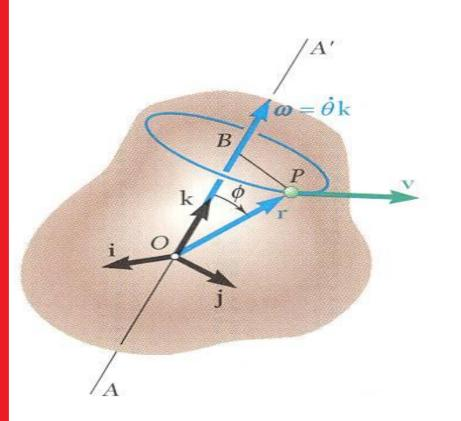
$$\vec{a} = \frac{d\vec{v}}{dt} = \frac{d}{dt} (\vec{\omega} \times \vec{r})$$
