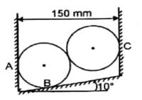
Solution: The system consists of two cylinders supported against three smooth surfaces at A, B and C. Let R<sub>A</sub>, R<sub>B</sub> and R<sub>C</sub> be the reactions at three supports. The FBD of the system is shown.
