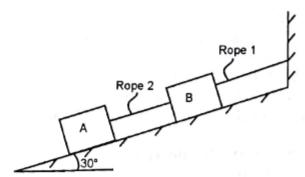
**Solution:** The system has two bodies viz blocks A and B which are externally supported by smooth surfaces offering reactions  $R_A$  and  $R_B$  and a rope (1) giving reaction  $T_1$ .
