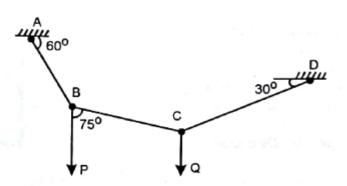
**Solution:** Isolating joint B of the string. Let  $T_{AB}$  and  $T_{BC}$  be the tensions in the string portions AB and BC respectively.
