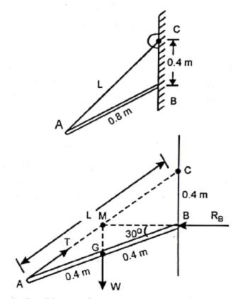
The weight W acts through the rod's C.G. Since the system has three forces in equilibrium, the forces should be concurrent. Let M be the point of concurrence of R<sub>B</sub>, T and W.
