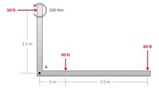
Q5. For a given force system find the resultant in magnitude and direction. Also find the equivalent resultant force and couple moment acting at A. (Forces are in KN and distance in m)
