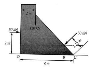
Q8 Replace the given force system by two parallel forces at B & D.
