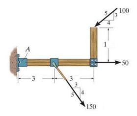
Q6 Determine resultant of given force system in magnitude and direction and locate it with respect to point 'A' Also find x and y intercept of resultant
