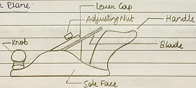
Bron Jack Plane is a general-purpose woodworking bench tool. It consists of Knob, Lever Cap, Adjusting Nut, Sole Face, Blade and handle. The Sole Face is the bottom part of the stock which is perfectly machined-flat. It is generally used for shaving off layer of wood to correct the thickness of the material. The thickness can be changed by adjusting the angle using the Nut and setting the blade at correct angle.
