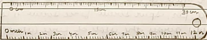
Steel Ruler or steel scale is a measuring tool which is one of the most important instrument. As the name suggests, its made from stainless-steel. The gradations are in cms & inches. The scale is available in different sizes which include 6 inches, 12 inches & 24 inches.
