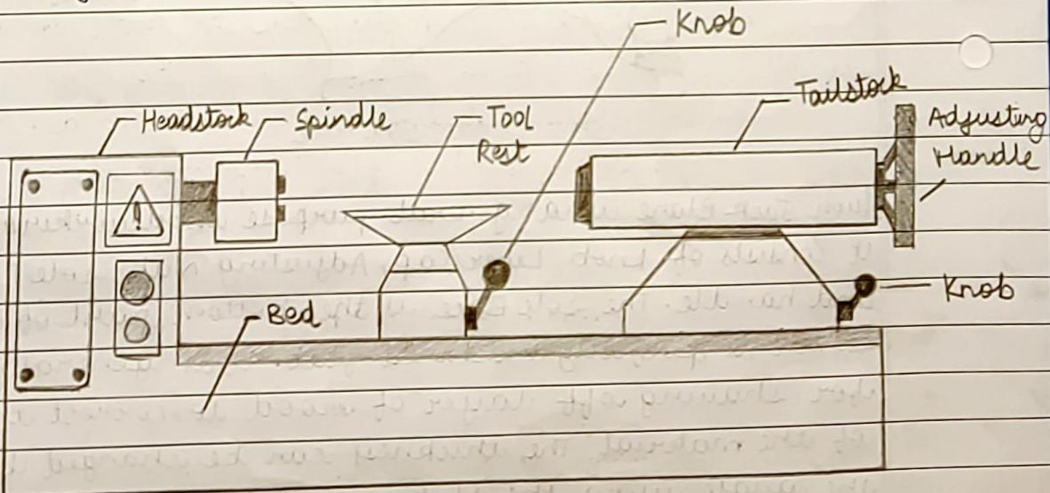
The Lathe Machine is an ancient tool. At the very early stage this machine was developed around 1300 BC at that time there were not so many parts except headstock & tailstock. It has evolved since then, a modern wood turning lathe machine consists of a iron bed, Headstock, Tailstock, spindle, Tool rest, adjusting knobs and speed controller.
