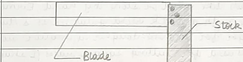
A Try-square is a woodworking tool used for making or checking 90° angles on pieces of wood. It is considered one of the essential tools for woodworking. It consists of blade & stock which are joined together by the means of rivet joint at an angle of 90°. The stock also has a clearance groove to take sharp edges while measuring 90°.
