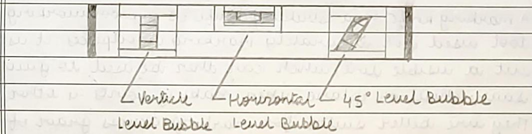
A spirit level or simply a bubble level is measuring instrument which is designed to indicate whether a surface is horizontal or vertical. A traditional carpenter's spirit level looks like a short plank of wood & often has a wide body to ensure stability. In the middle of the spirit level is a small window where the bubble in tube is mounted. It is often accompanied by a vertical or  $45^\circ$  level indicator.
