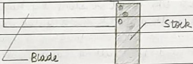
A Try-square is a woodworking tool used for making & checking  $90^\circ$  angles on pieces of wood. It is considered one of the essential tools for woodworking. It consists of blade & stock which are joined together by the means of rivet joint at an angle of  $90^\circ$ . The stock also has a clearance grooves to take sharp edges while measuring  $90^\circ$ .
