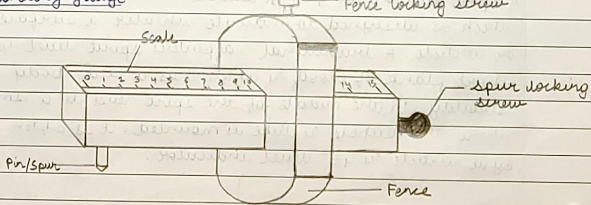
It is used for marking one parallel line at a time. It consists of Fence, pin, spur screw, fence screw & scale. The scale stem slides across the slot of fence (stock). Graduations are made in the form of a scale. The thumb screw is used for locking the ~~stem~~ screw in place. It is used in joinery & sheet metal operations.
