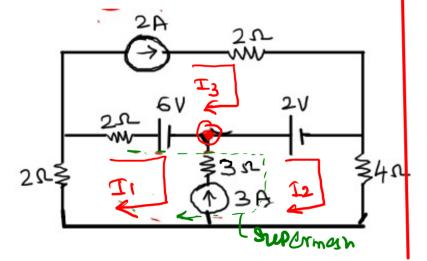
⇒ 2A current source on uncommon branch of mesh-3. ∴ T3 = 2A
