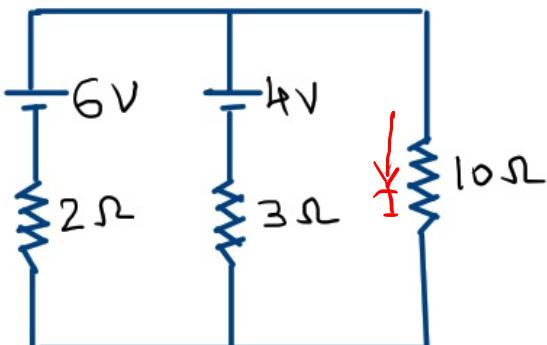
⇒ Consider 4V source in the circuit & replace 6V source by its internal resistance
