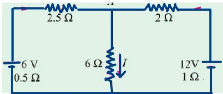
→ Consider 6V source in the circuit & replace 12V source by its internal resistance.
