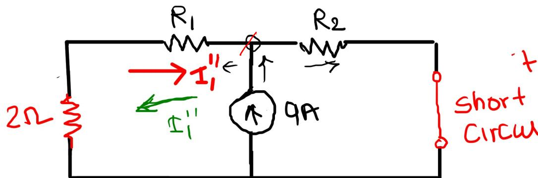
$$I_1' = \frac{R_2 \times 9}{R_1 + R_2 + 2} \quad (\leftarrow)$$
