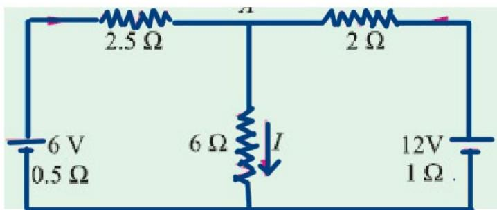
→ Consider 12V source in the circuit & replace 6V source by its internal resistance.
