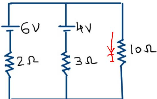
⇒ Consider 6V source in the circuit & replace 4V source by its internal resistance
