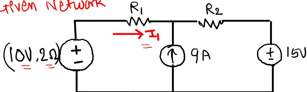
1. Consider 10V source in the circuit and replace 9A and 15V by their internal resistances
