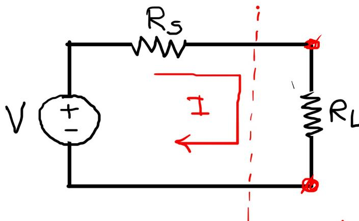
$$I = \frac{V}{R_s + R_L} \quad \dots \quad \textcircled{1}$$
