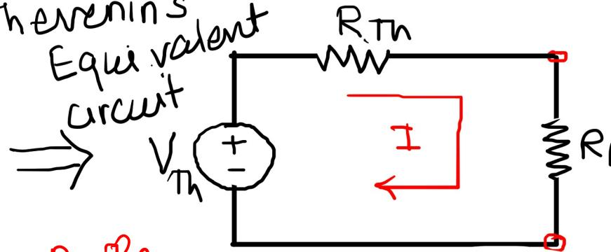
$$V_{RL} = \left( \frac{R_L}{R_L + R_{th}} \right) V_{th}$$
