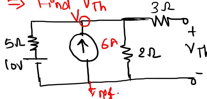
$$V_{Th} = V_{3\Omega} = V_{2\Omega} = V$$
