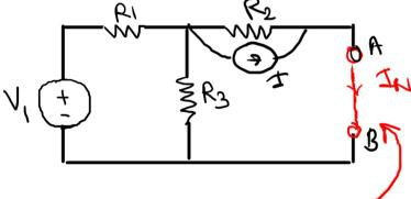
2. Find IN i.e. the short circuit current between the terminals (A-B) from where the load is removed, using any suitable method (mesh, nodal, source transformation etc...)
