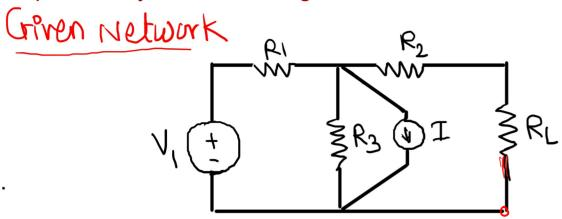
1. Remove load resistance RL from the given network
