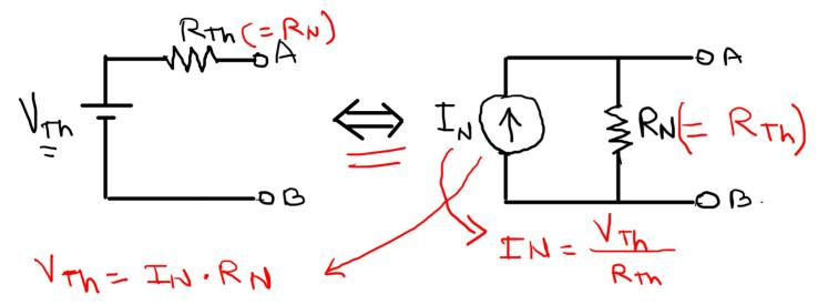
Norton's equivalent circuit can be obtained by applying source transformation to Thevenin's equivalent circuit.
