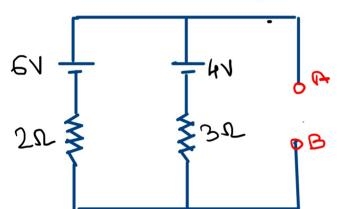
Mesh 0 mesh Analysis. Mesh  $2I_1 + 6 - 4 - 3(I_1 - I_2) = 0$  $5I_1 - 3I_2 = 0$  --- 0
