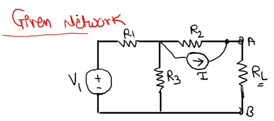
1. Remove the load RL from the circuit
