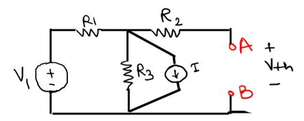
2. Find Vth i.e. the open circuit voltage between the terminals (A-B) from where the load is removed using any suitable method (mesh, nodal, source transformation etc..)
