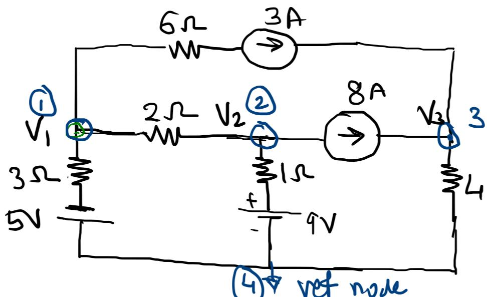
$\Rightarrow$  Type = 2  $\Rightarrow$  Voltage Source without series resistance appearing between Non-reference and reference node.
