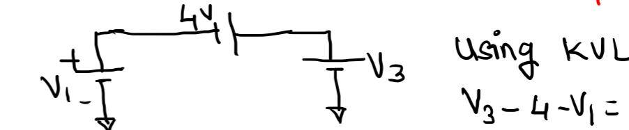
$$V_1 - V_3 = -4 \quad \dots \textcircled{1}$$
