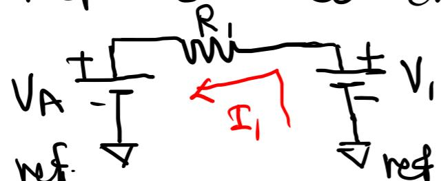
Using KVL →  $V_1 - I_1 R_1 - V_A = 0$
