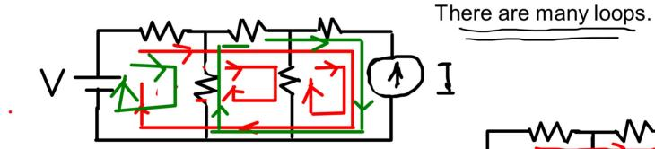
**Mesh** It is a loop which does not have loop inside it. Only loops marked with green are Mesh. The loops marked with red is not a Mesh.
