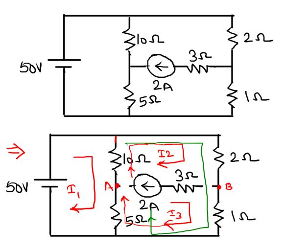
⇒ CUMPENT Source 2A applas on Common branch of mesh @ 2B So its supermesh case
