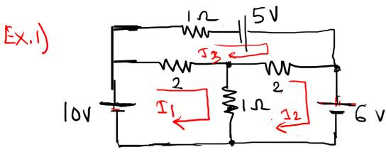
$\Rightarrow \text{ Identify mesh § mork} \qquad \Rightarrow \text{ Identify mesh § mork} \\ \text{mesh (urrent)} \\ \Rightarrow \text{ kul to mesh (I)} \\ 1D - 2(I_1 - I_3) - 1(I_1 - I_2) = D \\ 3I_1 - I_2 - 2I_3 = 10 - - (I) \\ \Rightarrow \text{ kul to mesh (I)} \\ - 2(I_2 - I_3) - 6 - 1(I_2 - I_1) = D \\ I_1 - 3I_2 + 2I_3 = 6 - - (2) \\ \end{cases}$
