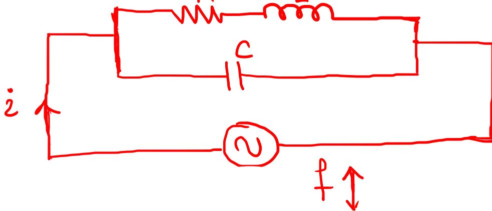
→ in parallel resonance circuit
