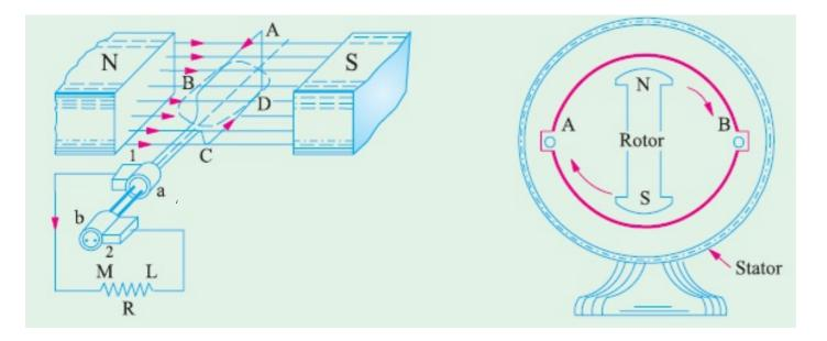
The amount of EMF induced into a coil cutting the magnetic lines of force is determined by the three factors.
