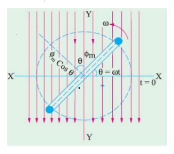
Rectangular coil, having N turns and rotating in a uniform magnetic field, with an angular velocity of  $\omega$  radian/second.
