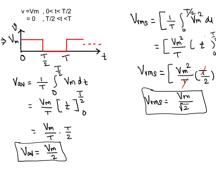
Example-7: Find the RMS value of the current indicated in the following waveform.
